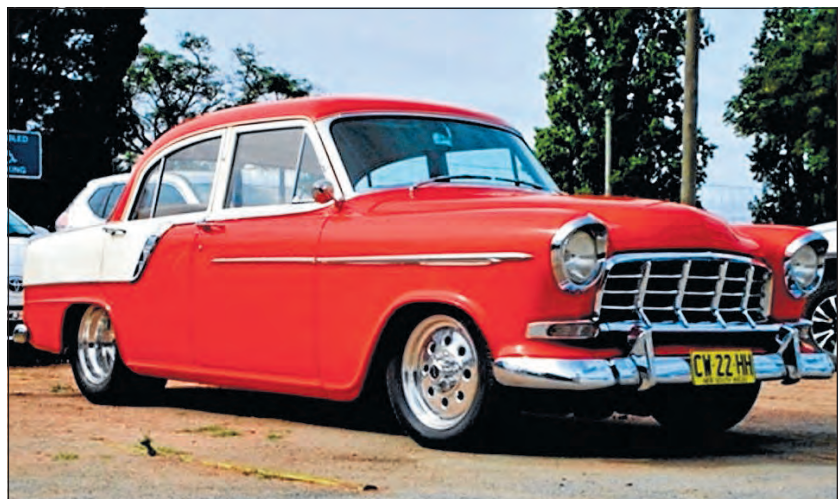
Colin Pettigrew's 1959 FC Holden, originally purchased 22 years ago, spent six months as the family car before being stored. Colin started working on it six years ago, stripping it back and totally rebuilding it in his shed, finishing it in time for this year's Rod Run. Photo supplied.
